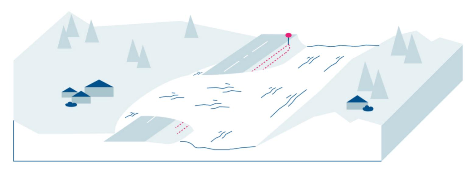
The river banks, when subjected to intense floods, can suddenly give way, producing catastrophic consequences. The deformation is a gradual process: it can be intercepted in time. Spider Bank is a system that monitors the state of the river banks using patented fiber optic technology. It allows to understand if there is a potential danger of collapse during floods.
